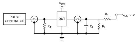
$R_T = Z_{OUT}$  of pulse generator (typically 50  $\Omega$ )
