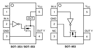
Figure 1. Pinout
